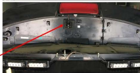
Strobe light wiring routed over the sealing foam compromising its ability to prevent air leakage
